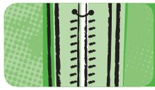
**4.** Slide the deckle into the basin. Put some pulp onto the screen and, still holding the deckle underwater, gently move it back and forth to get an even layer of fibers on the screen.
